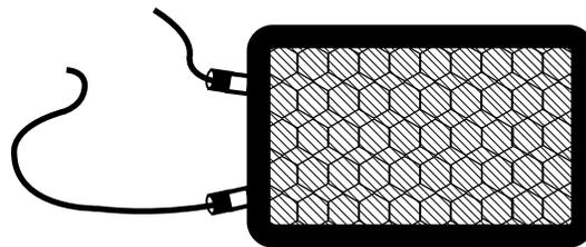
**8** Let the solder cool completely for 10 minutes. Gently pull on the wires to make sure that both are securely attached.
