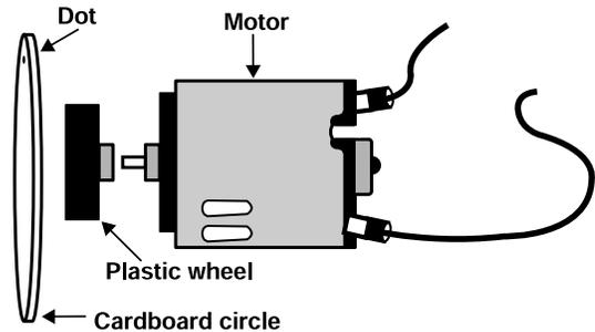
**11** Mark a small dot on the edge of the cardboard wheel. This dot will be used as a frame of reference to measure the speed that the wheel is spinning.
